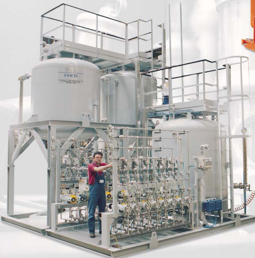
Zirku Gas Project - United Arab Emirates Glycol and Corrosion Inhibitor Injection Package. Customer: Technip Geoproduction - France
