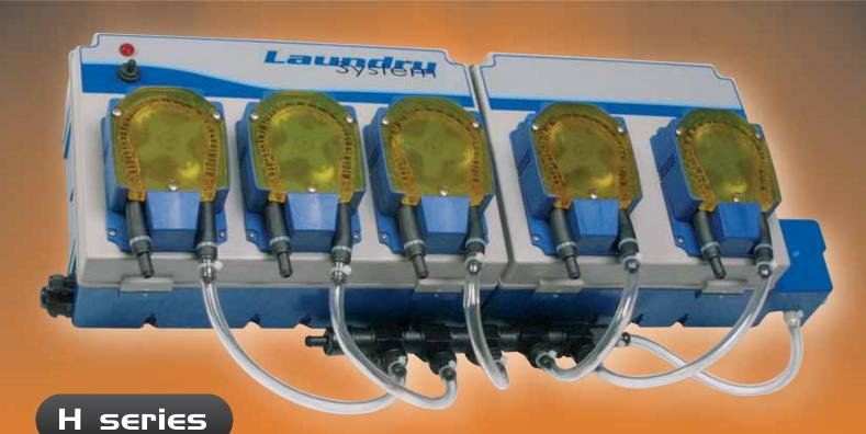
Pumps 2 to 7 • Flow rate 30 lt/h (500 ml/min) - 60 lt/h (1000 ml/min) - 90 lt/h (1500 ml/min) - 120 lt/h (2000 ml/min) Power supply 100 to 240 Vac 50-60 Hz • Power consumption 100 W max • 6 Input signals 20 to 230 Vac or 150 to 230 Vac
