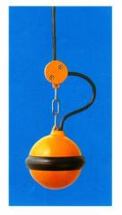
Model RF-5 is an economy float switch which can detect upper/lower limit water levels with a single float. The snap on-off action ensures stable pump operation in the clean or waste water containing suspended solids or oil and fat.
